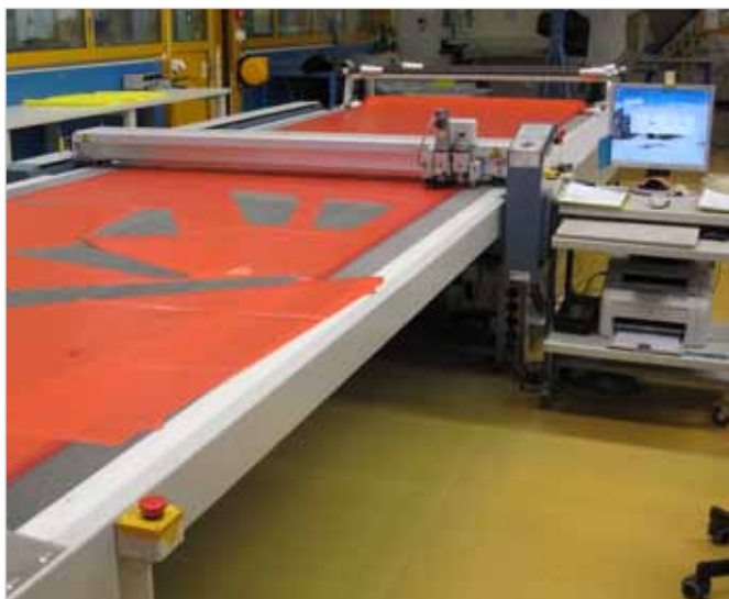
Cutting of carbon prepreg in the clean room.
